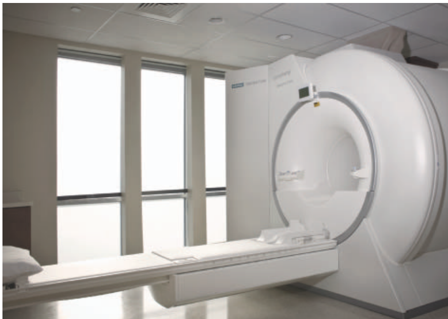
Figure 3 • Large amounts of natural daylight in the imaging room can help reduce patient anxiety, as well as lighting costs.
